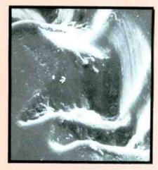
A disc with high groove modulation, as found in many modern recordings. Such modulation would be almost impossible to trace properly. (magnified 2000X)
