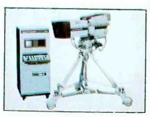
The HDTV camera was produced by Sony for the mentioned demonstrations. It is capable of more than 1200 lines resolution
