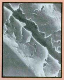
A 45 rpm disc shows peeling of the outer shell of polystyrene material after backcueing 10 times with a spherical tip. (magnified 10,000X)
