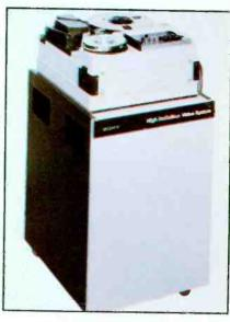
The HDTV system demonstrated included a modified portable 1-inch, C-format machine that provides 3-channel component recording of R, G and B. Here the higher tape consumption reduces the normal 1-hour operation to about 20 minutes.
