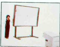
Here is a 100-inch (diagonally) projection screen monitor that operates on the 1125-line signal of high definition. The advantages are that it has none of the resolution limitations of shadow mask or Trinitron stripe picture tubes.
