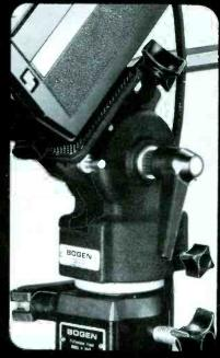
Measuring just 5" x 5" x 5" (excluding handle), this light-weight, fluid-damped type tripod head accommodates a wide range of cine/video cameras. It pans smoothly a full 360°, tilts 45° up and 90° down, with a safety detent at -45° and features separate pan and tilt locks.
